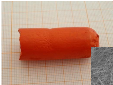
SbSI ethanogel consisted of nanowires
