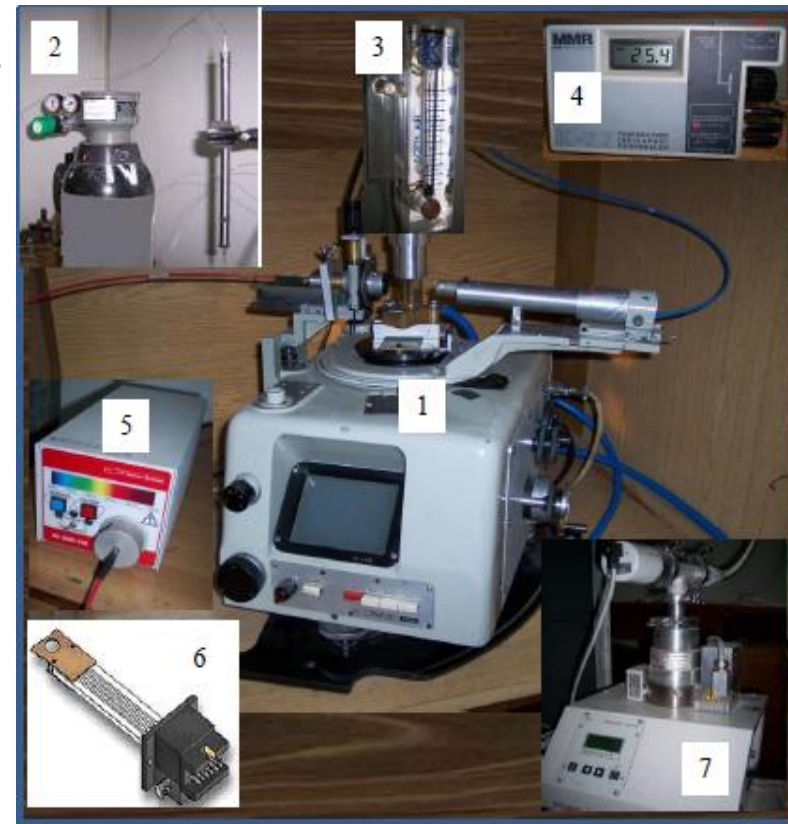
Picture of the experimental set-up for spectrogoniometric measurements performed at various temperatures 1 – goniometer, 2 – cylinder with nitrogen gas and filter, 3 – rotameter, 4 – temperature controller, 5 – light source, 6 – refrigerator, 7 – vacuum pump)
